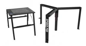
Large staging risers are often used as camera platforms. However, as an operator shifts footing, the camera and tripod may shake producing an unstable video image. When multiple shooters are on these shaky staging risers or camera are zoomed in, the problem is magnified. The Spider Pod features a separate tripod riser and standing platform eliminating camera shake caused by the camera operator. Tripod riser supports up to 200.0 lbs., the standing platform up to 300.0 lbs.
