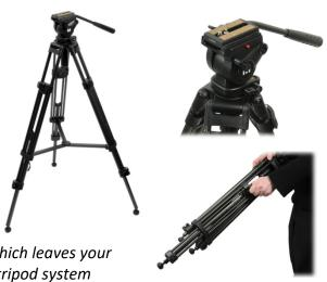
Its 2-stage leg design allows you to adjust the height of the tripod from 27.6" to 59". A middle spreader and passive counterbalance provide enhanced stability to the entire system. The VT-4000 also has separate pan and tilt locks, and a bubble level for precision leveling. The fixed counter-balance spring incorporated in the head will help with smoother tilt movements.
